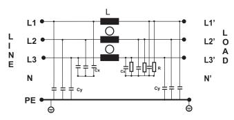
Technical Specification Max Rated Voltage 3x 440/250 VAC Operating Frequency DC to 50/60Hz Rated Current 8A to 280A @50°C High Voltage Test -
