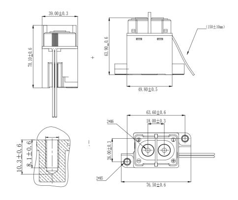
\*Note: The wire size is 20AWG-22AWG, diameter 1.5mm including insulation layer
